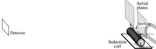
Heinrich Hertz used apparatus resembling what is shown in this diagram to test for the existence of a new type of radiation.
