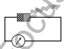
Of the following, which could represent the p-n-junction device shown in the above circuit diagram?
