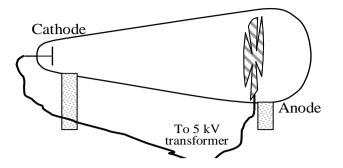
In the latter part of the 19<sup>th</sup> century, Sir William Crookes designed a special cathode-ray tube that looked similar to this in order to identify certain properties of cathode-rays.
