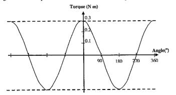
(a) A current of 600mA is travelling through the windings when the coil is parallel to the magnetic field. The coil consists of 200 turns of wire and has an area of 1.5 x 10<sup>-3</sup> m<sup>2</sup>. Use this information and the graph above to calculate the magnetic field strength.
