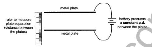
She measured the electric field strength E for different values of plate separation d, then plotted E against d.
