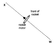
When the rocket reaches point X, the rocket motor is fired for a short time straight ahead (in the direction the rocket is pointing), until the rocket reaches point Y, when the motor is turned off. Assume that the rocket motor produces constant thrust (force) while going from X to Y, and that only a very tiny amount of fuel is used.
