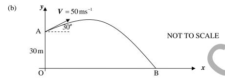
A body is projected from a point 30 metres above level ground with velocity  $50~{\rm ms}^{-1}$  and inclined at an angle of  $30^{\rm o}$  to the horizontal as shown in the sketch. The body lands on the ground at the point B.
