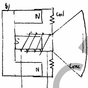
A loudspeaker changes electrical energy to sound energy using the force on a current-carrying wire in a field  $B$ . (See Fig.).
