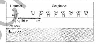
The data from the geophones are analysed and the arrival times of the direct and refracted waves that reach each geophone are recorded. These data are shown in the graph on page 33. On the graph, a circle represents the arrival of the first wave to reach a geophone, and a square represents the arrival time of the second wave to reach a geophone. The points on the graph associated with the direct seismic wave and the refracted seismic wave are shown.
