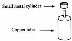
Yet a small magnet of identical dimensions takes much longer to fall through the tube.
