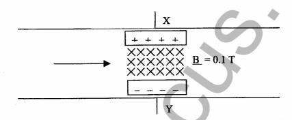
Calculate the potential difference across the parallel plates, XY, required to allow the electron to pass undeflected through the electric and magnetic fields. The distance between the plates is 10 cm. 3
