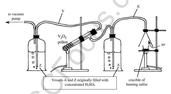
(i) Evaluate the feasibility of Ken's apparatus to produce sulfuric acid ignoring safety issues
